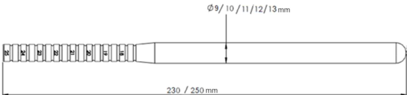
The prosthesis is sterile and single use. It is available in different sizes consisting of five diameters and two lengths. Please see the diagram above. Each prosthesis comes with two different extender sizes to adjust the length of the prosthesis according to the corporal length of the patient. The extenders are easy to connect/assemble.
